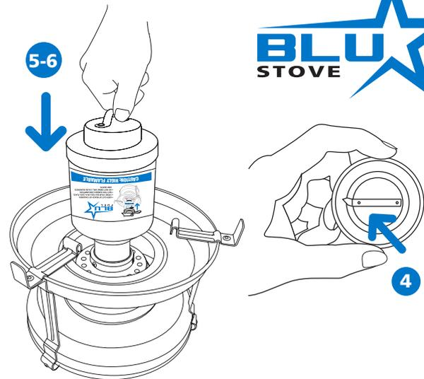
4. On the inside of the shutoff cap is a punch pin.
